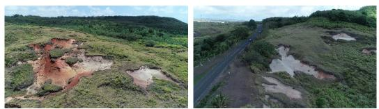
Aerial photographs (from UAV) of rainfall-induced shallow slope failures in Inarajan
