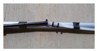
**Step 4.** Fully extend the telescoping pole top end and tape the nozzle to the top end on the pole.
