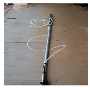
**Step 7.** Use electrical tape again to attach the trigger end of the wand to the pole four feet up from the base of the pole.
