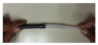
**Step 3.** Insert the other half of the polyethylene tubing midway into clear vinyl tubing connected to the nozzle half of the spray wand. Repeat process on other end of the sprayer wand. Use zip ties to secure the tube ending.
