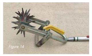
*Scuffle hoes with spiked wheels (crumbler).* These go a step further. They have a row of spiked wheels mounted behind the scuffle hoe blade (Figure 14). As
