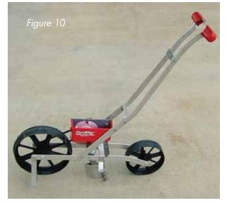
Some seeders add a fertilizer hopper to meter granular fertilizer into the soil while planting. Many have an arm with a tooth on it that can be dropped down to mark the correct location for the next row. Additional optional seed plates for other crops may be available.
