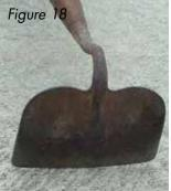
shape such as the fingers and bows on a rake or the blade and attaching rod on a hoe. Forging greatly increases the strength of the steel in the direction of elongation, which usually is the direction of most force in garden use.
