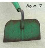
rods welded to the head to make the bow that fastens to the handle. Similarly, the blade of a hoe is stamped out and a rod with a handle socket is welded to the blade. The welding process weakens the tool, but if you want a tool for only occasional light-duty use, an inexpensive welded tool probably will suffice. Never pay a premium price for a welded tool.
