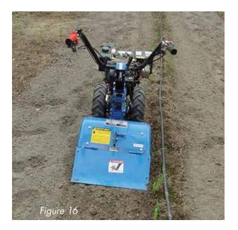
**Rotary tillers**. Tillers can be effective at cultivating around crops, and the cultivation can usually be done at a higher ground speed than you would use for primary or secondary tillage (Figure 16). Be careful to use a very shallow depth setting when cultivating to avoid damaging crop roots. It is best to avoid walking on the cultivated ground since weeds will germinate and/or reestablish better in your footprints.
