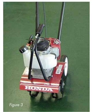
*Size.* Several companies offer small, hand-held rotary tillers, typically with 2-cycle engines (Figure 3). These little tillers have star-shaped sheet-metal blades instead of discrete tines. They are suitable for very light tilling such as cultivating small vegetable or flower gardens. They are narrow and can get into tight places. They will not till deeply, nor will they handle much surface trash. These small tillers are seldom a good choice for soil preparation prior to planting.
