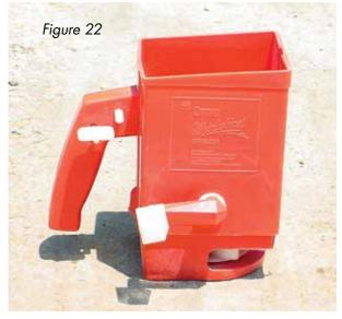
**Types of hand-cranked spreaders.** Several types of hand-cranked spreaders are available. The least expensive has a very small hopper and is held with one hand while cranking with the other (Figure 22). Larger units are carried on a strap around the operator's neck (Figure 23). These generally are of two subtypes. One type is designed to broadcast granules both right and left; the other type broadcasts primarily to one side.
