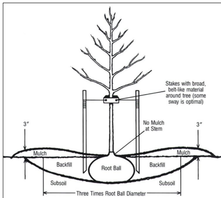
**Figure 27.** General hardware guidelines for tree installation
