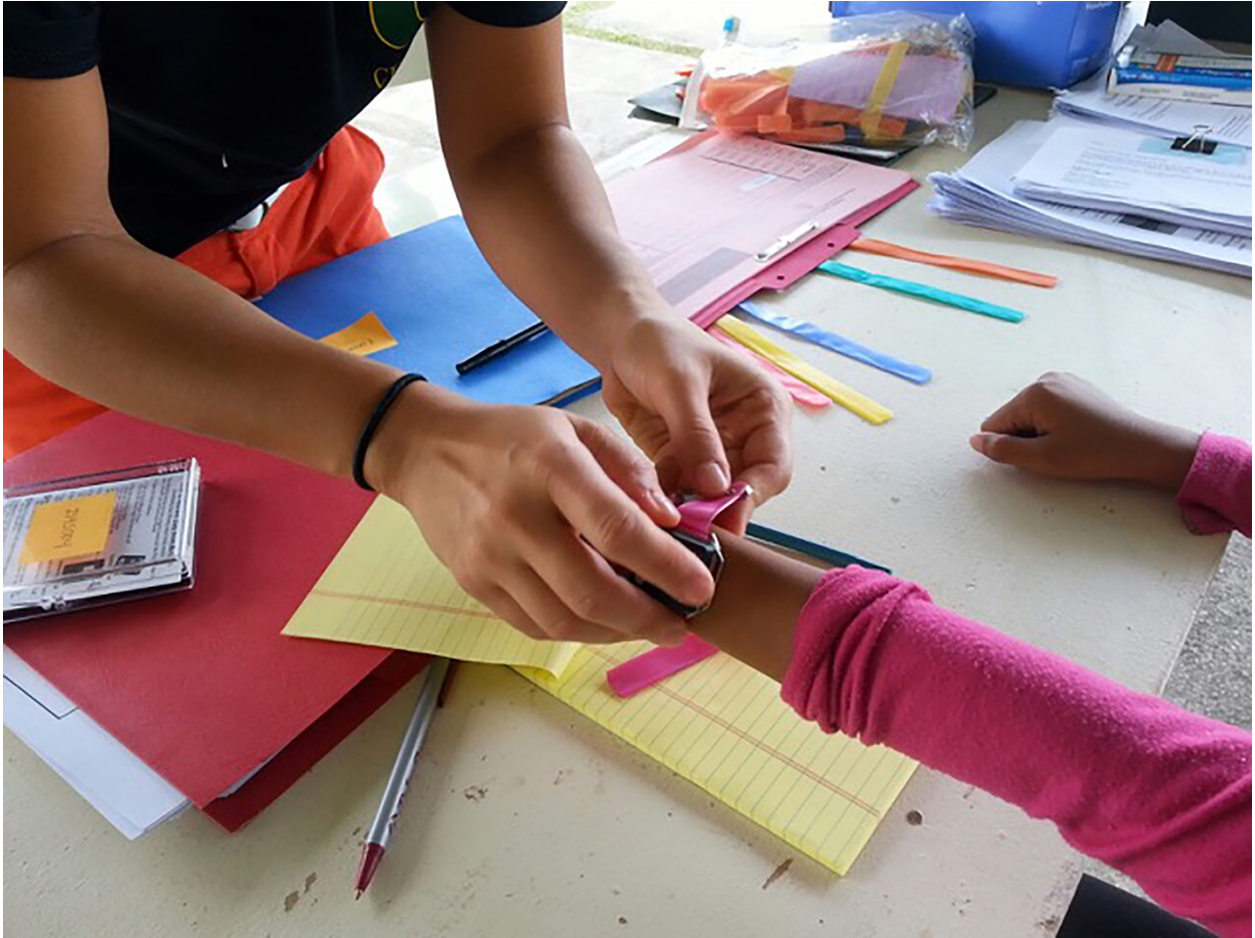
An “Actical” bracelet is placed on the wrist of a Children’s Healthy Living Program participant to measure physical activity.
