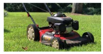
Figure 2. The blade of a rotary mower spins in a horizontal plane, striking and severing vertically growing leaf blades.
